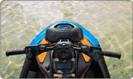
BRP Audio - Portable System (optional) The BRP Audio - Portable System provides higher-quality sound on and off the water featuring Concert, Ride and Home modes. Equipped with a heavy-duty mounting bracket.
